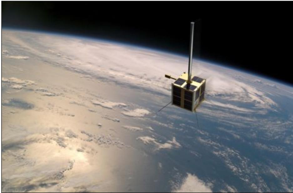
The Norwegian AISSat-1, launched Monday and depicted here in orbit, will improve marine safety in the High North by tracking vessels weighing more than 300 tons. The cube is 20 centimeters long on each side and weighs six kilograms. Image courtesy of the Norwegian Space Centre.
