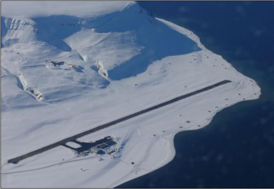
The runway at Svalbard Airport is built with flexible asphalt designed to withstand temperatures as low as minus 40° Celsius. But aerobridges can't reliably attach to planes due to frequent high winds, meaning passengers must walk outdoors to and from the terminal.
